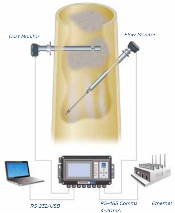
Figure 4: STACKFLOW 400 combined with a PCME dust monitor for integrated concentration and mass emissions reporting
