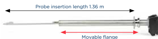
Figure 2: STACKFLOW 400 sensor with movable flange to locate the optimum measurement path
